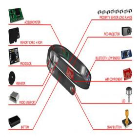
The Cicret uses a Pico projector to throw your mobile's screen into your arm. It also features eight proximity sensors which the bracelet uses to detect your finger position so as to feedback controls. This means you
