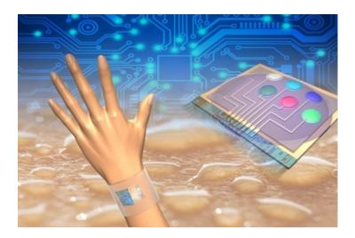
The researchers tested the device on 26 men and women who pedaled indoors on stationary bikes or ran outdoors on tracks and trails. Sodium and potassium in sweat could help check for problems such as dehydration and muscle cramps. Glucose could help keep track of blood sugar levels. Lactate levels could indicate blood flow problems, and skin temperature could reveal overheating and other problems.
