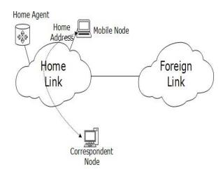
When Mobile Node leaves its Home Link and is connected to some Foreign Link, the Mobility feature of IPv6 comes into play. After connecting to Foreign Link, Mobile Node acquires an IPv6 address from Foreign Link. This address is called Care-of Address. Mobile Node sends binding request to its Home Agent with the new Care-of Address. Home Agent binds Mobile Node's Home Address with Care-of Address, establishing a Tunnel between both.
