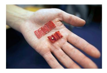
The new robot can unfold from an ingestible capsule and operate inside the stomach.
