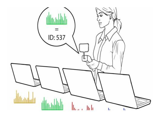
Radio frequency emission are considered incidental system noise in virtually all laptops, smartphones and other electronic devices, but scientists at Disney Research have found a way to use these spurious electromagnetic (EM) signals to uniquely identify even seemingly identical devices.
