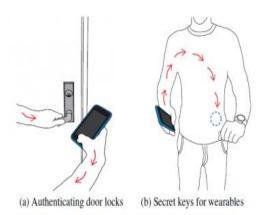
These "on-body" transmissions offer a more secure way to transmit authenticating information between devices that touch parts of our body — such as a smart door lock or wearable medical device — and a phone or device that confirms our identity by asking us to type in a password.
